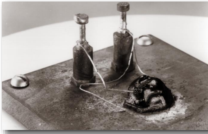
Transistor, 1950 @ Bell Labs
