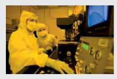
**INRF** is a 9,600-square-foot Class 100/1,000/10,000 cleanroom equipped with all the major tools for micro- and nanofabrication. **http://www.inrf.uci.edu/**
