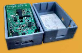
Electrical engineer Andrew Dylan Begey '18, project lead of the first MDP team, was responsible for designing the device's initial printed circuit board. "Our goal was to integrate several different commercial products all onto a single PCB and add more functionality, such as inductive battery charging and battery-level monitoring. In the end, two revisions of the device were completed and proved functional."
