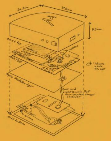
Above: The student team's design integrates the microcontroller, motion sensor, power and battery management, and inductive charging all onto a small wearable circuit board.
